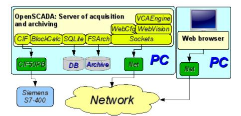
Рис. 6. Client access by means of the Web-interface. A place of the manager.
