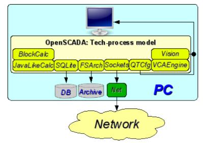
Рис. 9. The elementary mixed connection (model, demonstration, configurator...).
