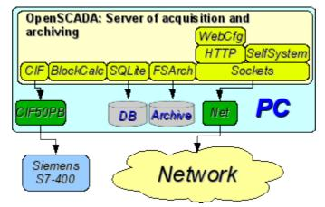
Рис. 3. Simple server connection.
