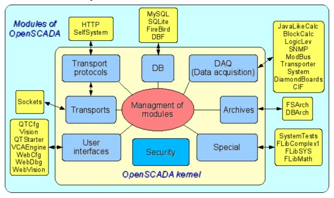
Рис. 1. The block scheme of OpenSCADA system
