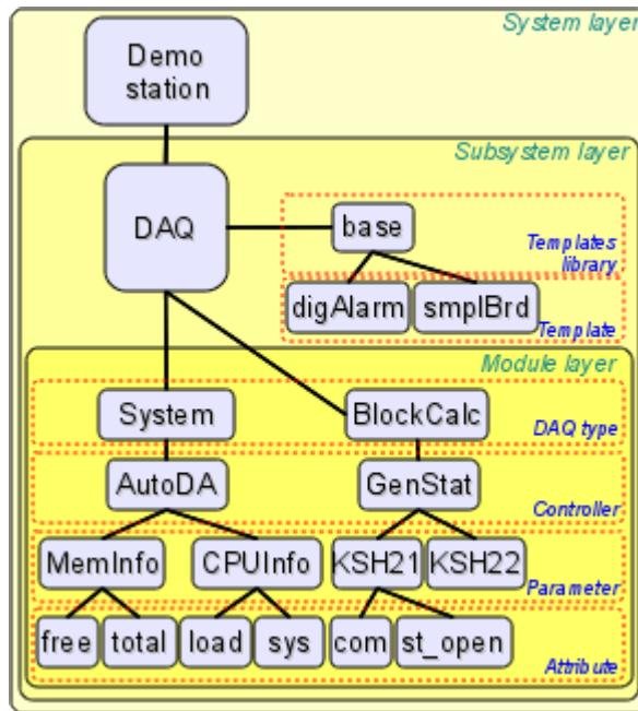
Fig. 4.5a. The hierarchical structure of subsystem "Data acquisition".
