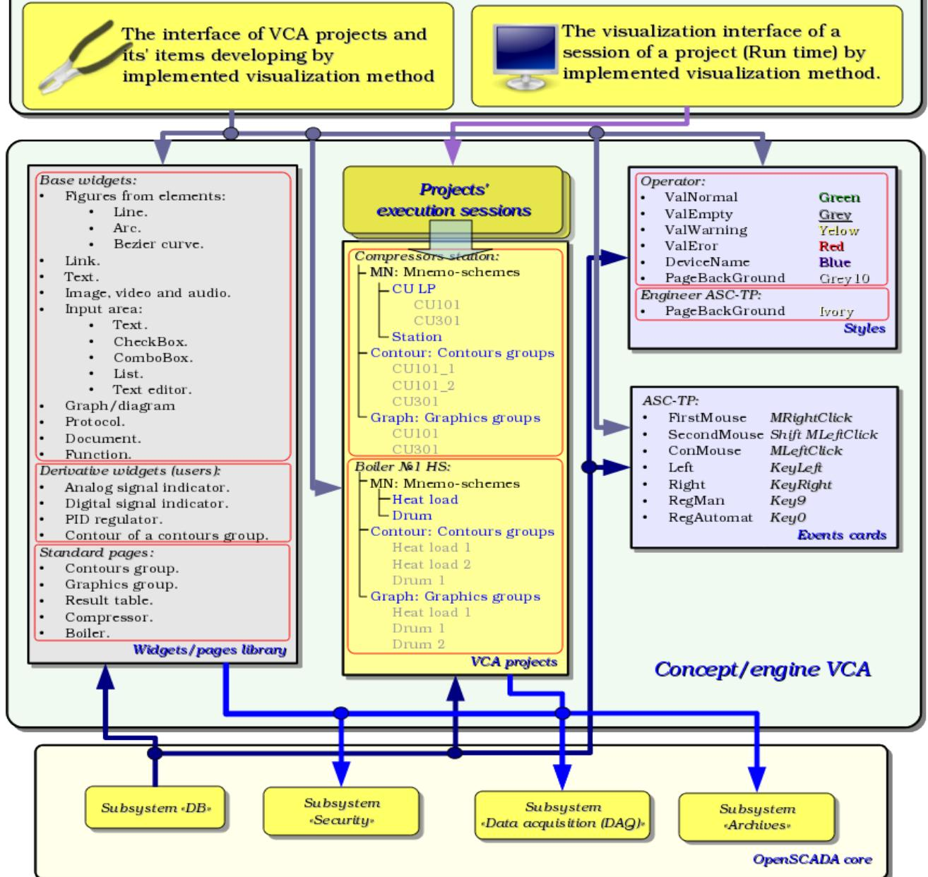
Fig.3 Generalized structure of the VCA.
