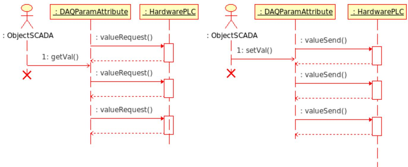
Fig. 3. Diagram of interaction sequence with asynchronous requests.
