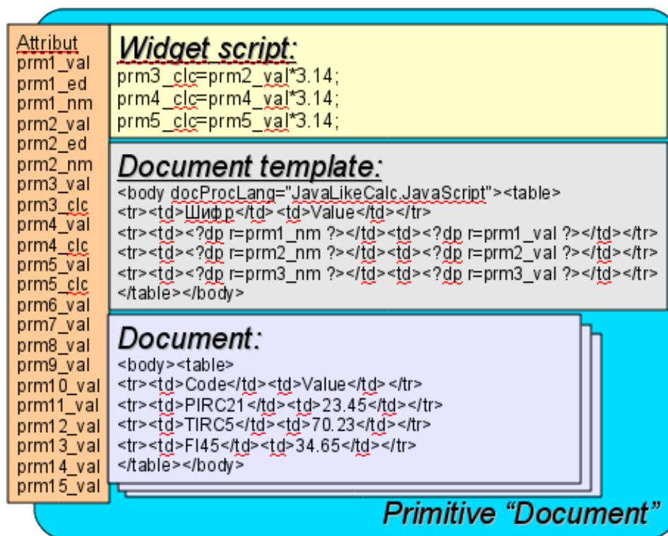
Fig. 3.8.7.a The block diagram of the primitive "Document".
