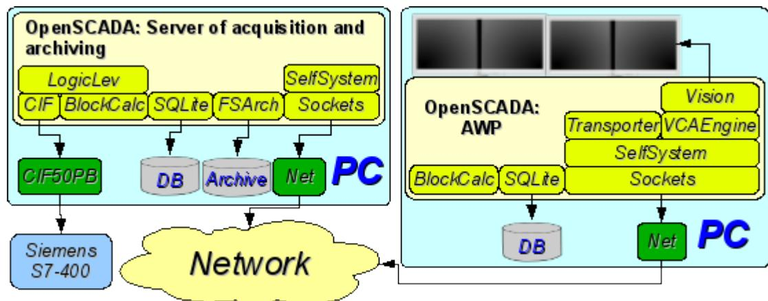
Fig. 3.5. The automated workplace (place of the manager/operator).
