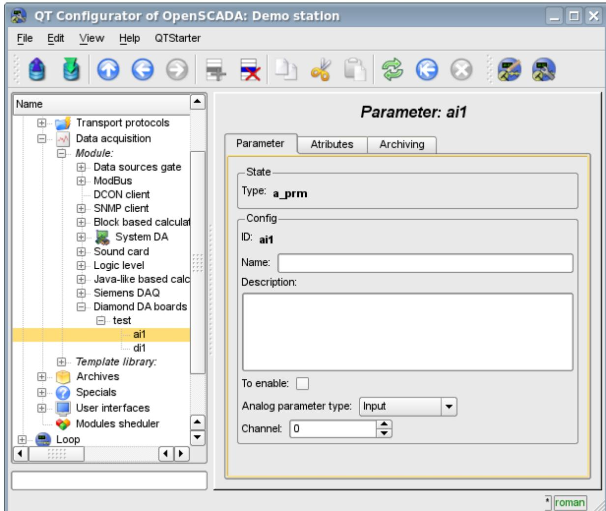
Fig.3. Tab of the configuration of analog parameters.
