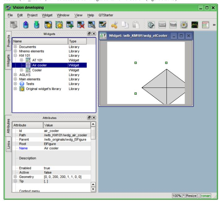
Fig. 5.3.2.3. Adding the inherited widget "air cooler".
