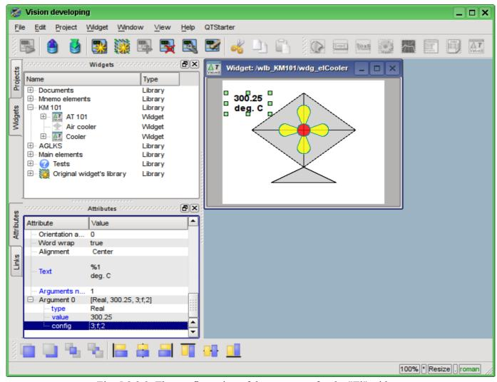
Fig. 5.3.2.9. The configuration of the argument for the "Ti" widget.
