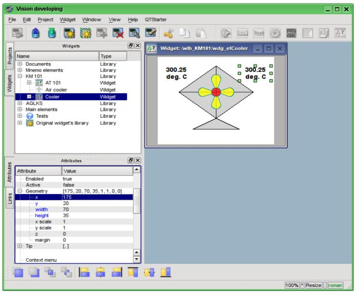
Fig. 5.3.2.12. Changing the geometry of the "To" widget.
