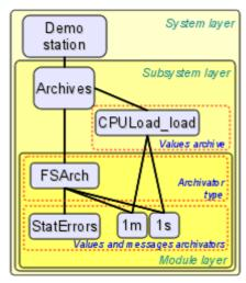
Fig. 4.6a. The hierarchical structure of subsystem "Archives"
