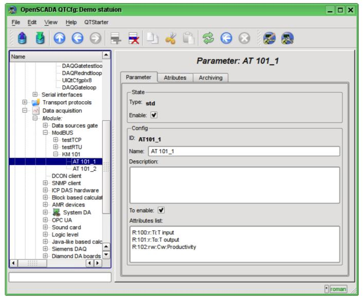
Fig. 4.1.6. Configuration page of the controller's parameter "ModBUS".
