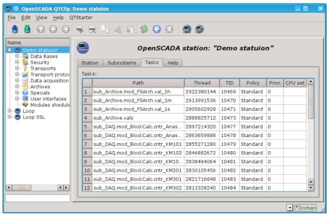
Fig 4c. "Tasks" tab of the main page of the configuration of the station.
