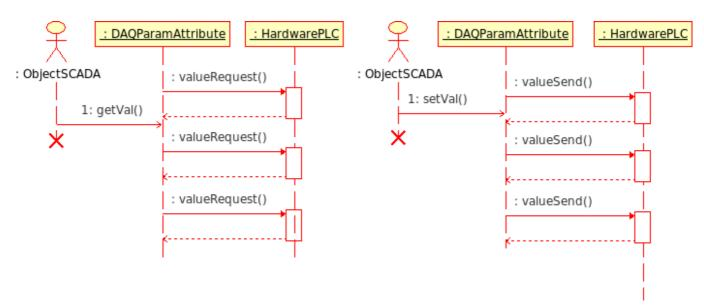
Fig. 3. Diagram of interaction sequence with asynchronous requests.
