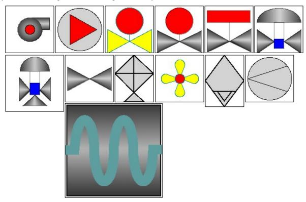
Fig.1. Elements representing technological devices from left to right and top to bottom: "Compressor", "Compressor 1", "Bolt", "Crane", "Ball crane", "Crane and position", "Three-positioned crane", "Valve" "Cooler", "Cooler", "Separator", "Diaphragma", "Zmejev hor".
