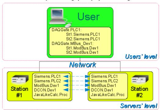
Fig.1. Horizontal and vertical redundancy.
