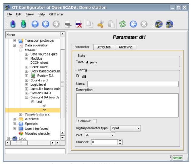
Fig.4. Configuration tab of digital parameters.
