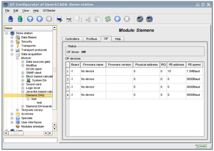
Fig.1. Configuration tab of CIF-boards.
