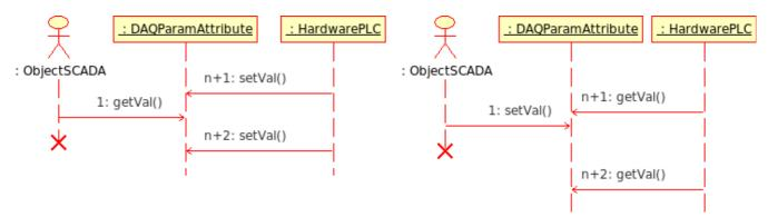
Fig. 5. Diagram of interaction sequence with the passive working mode.
