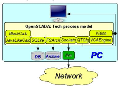
Fig. 3.7. The elementary mixed connection (model, demonstration, configurator...).
