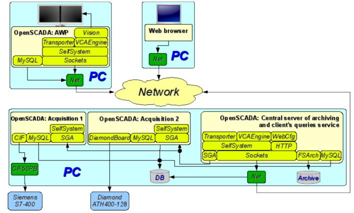
Fig. 3.8. The steady, allocated configuration.
