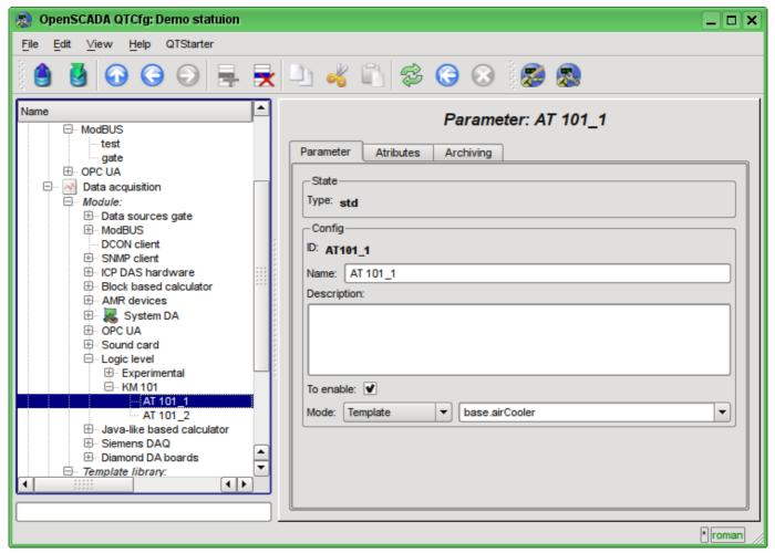
Fig. 4.2.4. Configuration page of the "LogicLev" controller's parameter.
