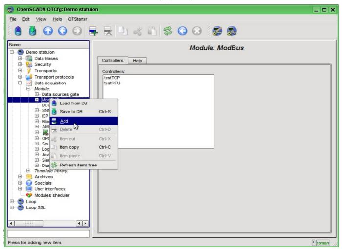
Fig. 4.1.1. Adding the controller in the "ModBUS" module of the subsystem "Data acquisition".
